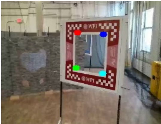
Fig. 4. window2 detection in runtime
