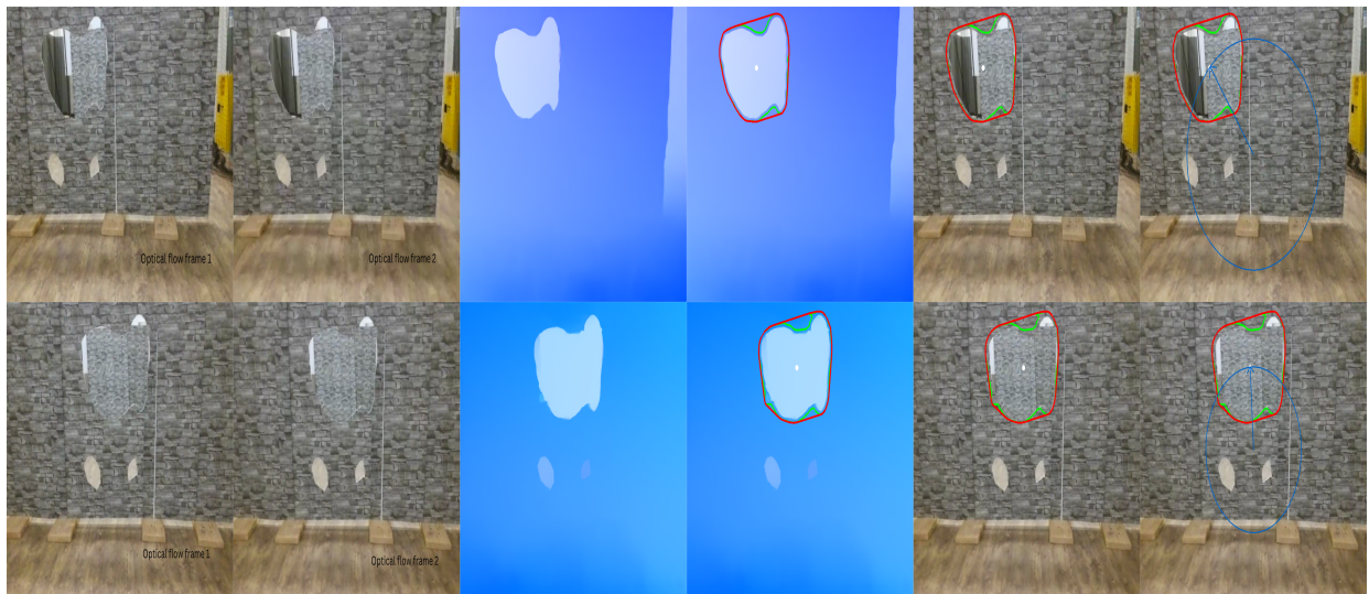
Fig. 9. Results from a real world run. Row 1: Flow estimation at the initial location, Row 2: Flow estimation after correction and just before going through gap. (Left to right: Frame 1, frame 2 used for flow, Optical flow, Gap contour and center identified on flow, Contour and center on frame, Distance between gap center and image center)
