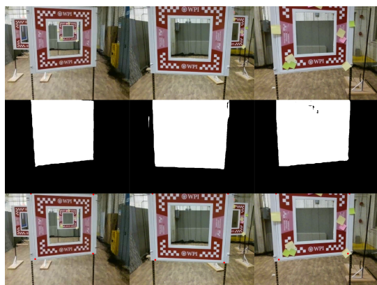
Fig. 4. Row 1: input image frames; Row 2: YOLOv8 prediction mask Row 3: Inferred corners after post-processing
