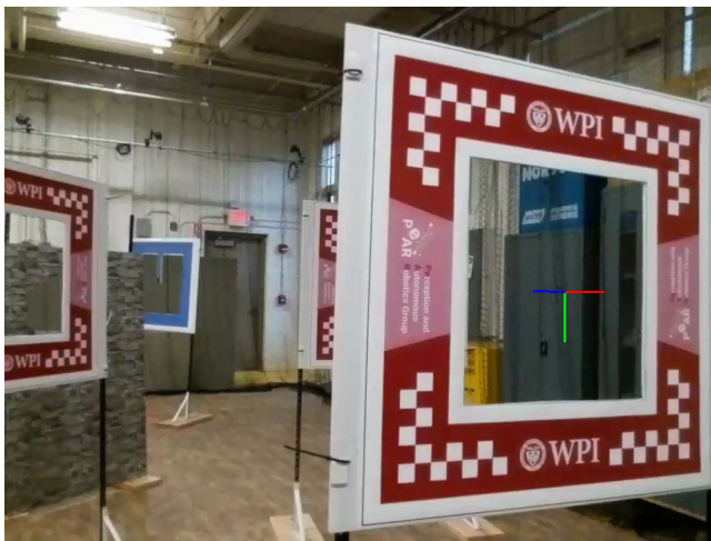
Fig. 11: "Reprojecting the Window center in drone camera frame"
