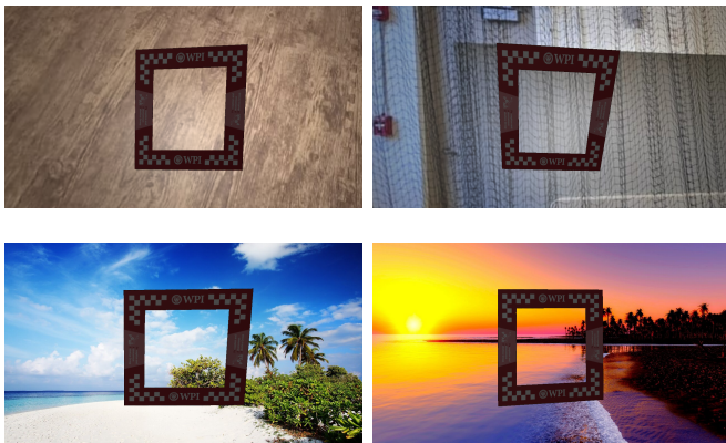
Fig. 3: RGB Images with applied homography and different backgrounds
