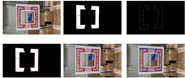
Fig. 9: Delaunay Triangulation pipeline
