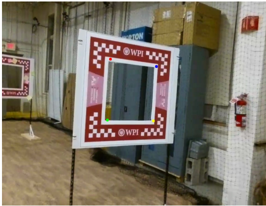
Fig. 8. Checker board pattern used for camera calibration
