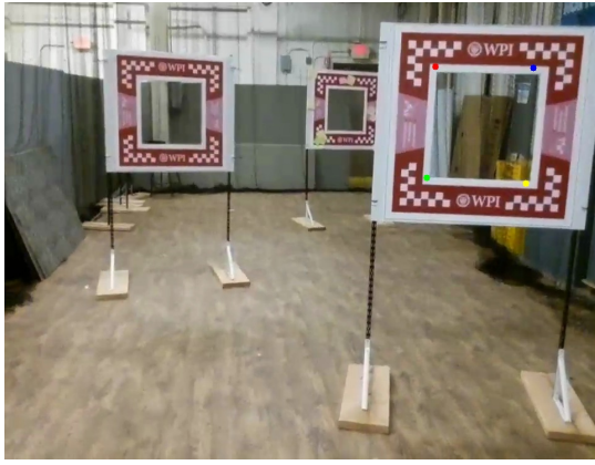
Fig. 7. Checker board pattern used for camera calibration
