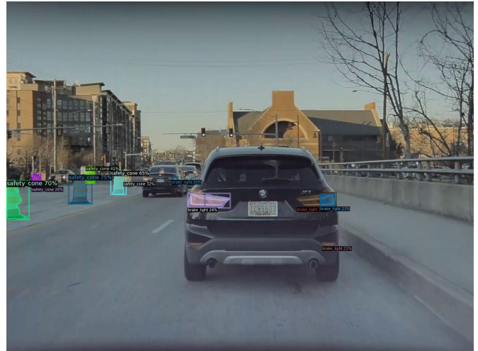
Fig. 8. Detection of Safety cones and braking light using Detic
