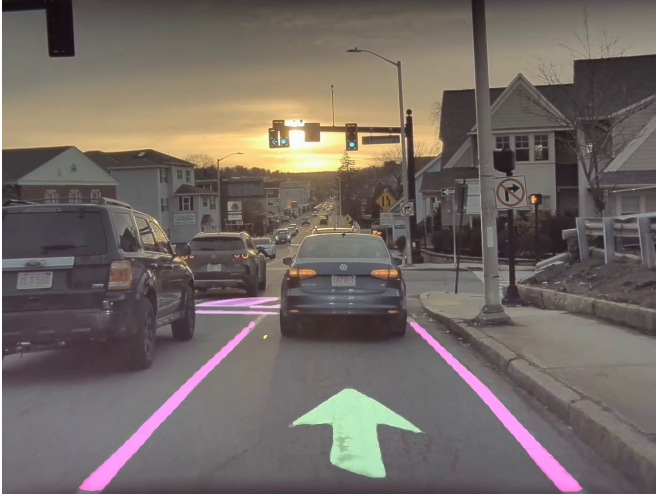
Fig. 5. Detection of road arrows using Mask RCNN
