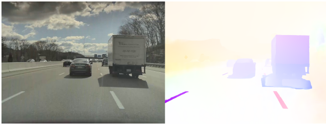
Fig. 9. Image (left) and Optical Flow(right)
