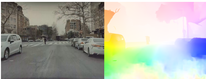
Fig. 10. Image (left) and Optical Flow(right)
