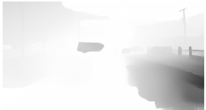
Fig. 23. Grayscale Flow for Parked and Moving Vehicle Estimation
