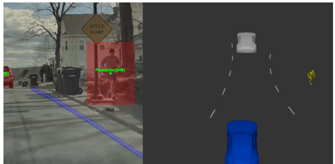
Fig. 19. Pedestrian Pose estimation and Speed Limit Edge Case
