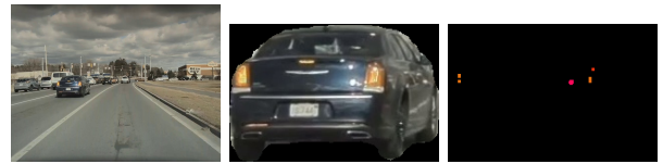
Fig. 15. (Left to Right) Original Image from Scene 3, Isolated masked car Image and the filtered image to identify brake lights
