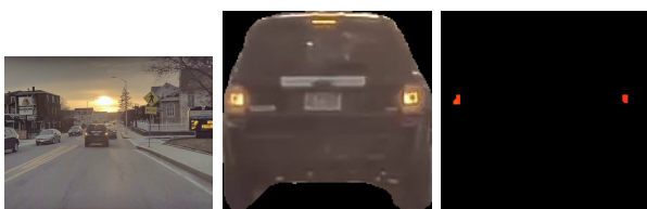
Fig. 14. (Left to Right) Original Image from Scene 11, Isolated masked car Image and the filtered image to identify brake lights
