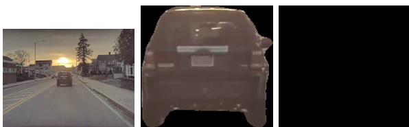
Fig. 13. (Left to Right) Original Image from Scene 11, Isolated masked car Image and the filtered image to identify brake lights
