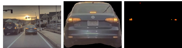
Fig. 10. (Left to Right) Original Image from Scene 11, Isolated masked car Image and the filtered image to identify brake lights
