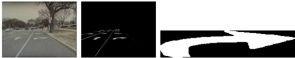
Fig. 7. (Left to Right)Original Image from Scene 7, Isolated signs on the road and the Resulting largest Contour obtained
