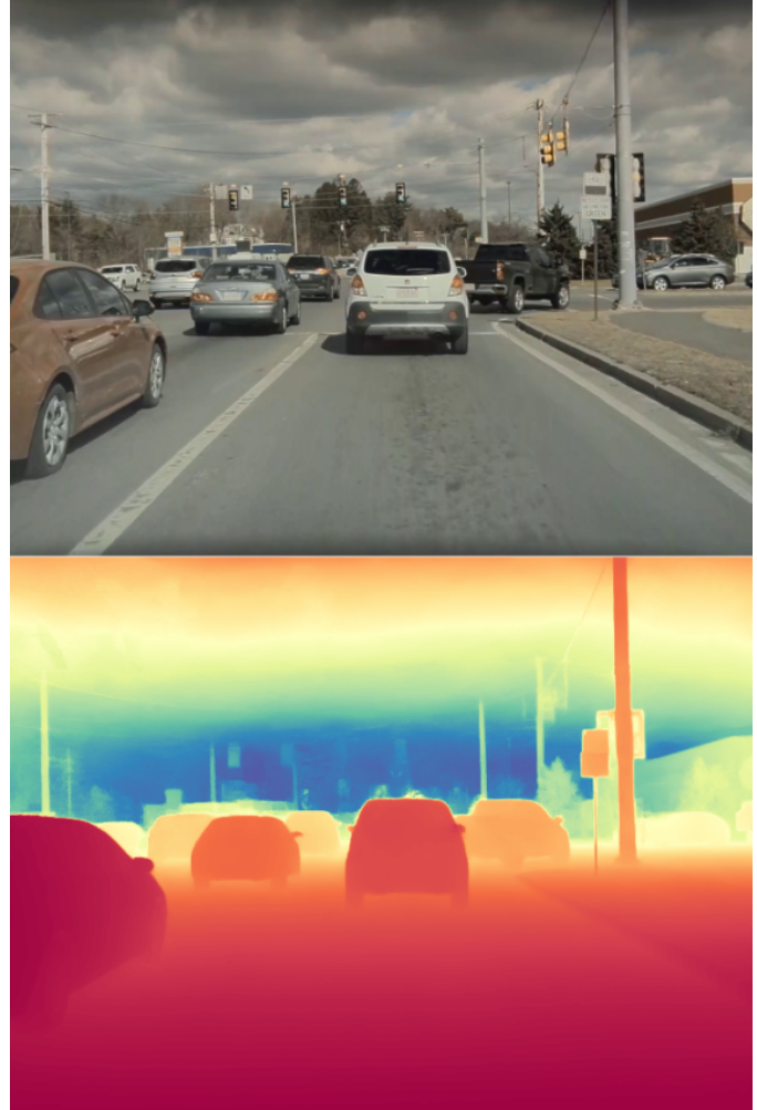
Fig. 1: Depth Estimation from Monocular RGB Image. Top shows the original image and Bottom shows the estimated depth.
