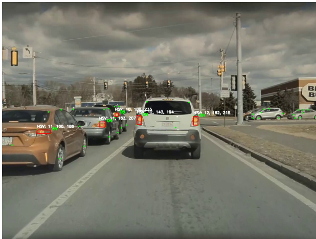
Fig. 9: "ON or OFF" visualization created to test our thresholds of detected tail light bounding box
