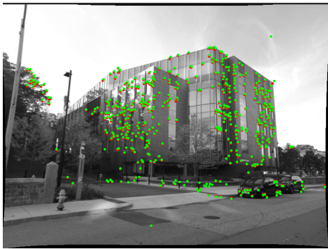
Fig. 6. Reprojected points after nonlinear triangulation.
