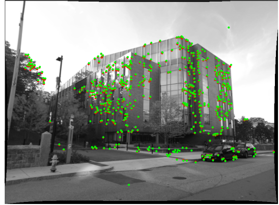
Fig. 5. Reprojected points after linear triangulation.
