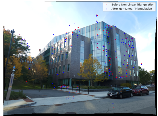
Fig. 5: Improvement in feature projection after non-linear PnP
