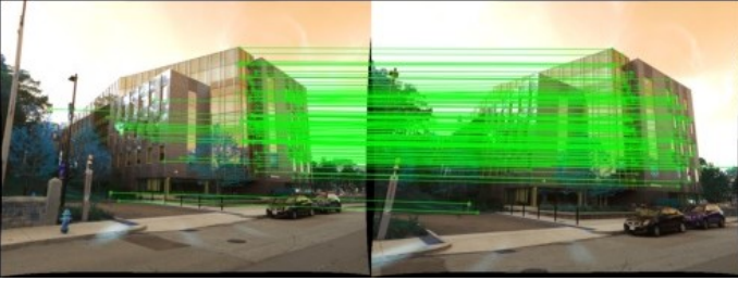
Fig. 4. Outlier Rejection - RANSAC (using Fundamental matrix)
