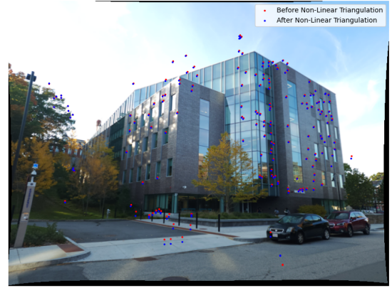
Fig. 5: Improvement in feature projection after non-linear PnP
