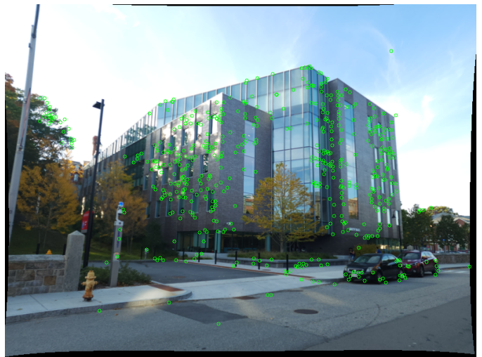
Fig. 6. Reprojection of linear triangulation depth points onto image 1
