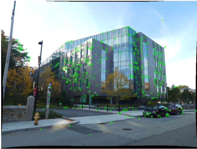
Fig. 9. Reprojection of non-linear triangulation depth points onto image 2
