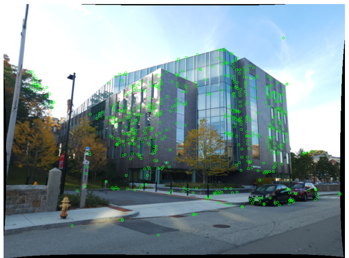
Fig. 8. Reprojection of non-linear triangulation depth points onto image 1
