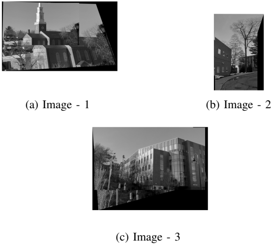
Fig. 13: Panorama Stitching for 2 images for each of the test set for supervised learning: Images aren't stitched as pure translation between the images is not learned by the model. The resultant homography matrices are estimated incorrectly
