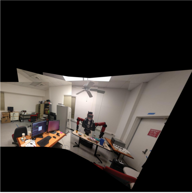
Fig. 8: Panorama Stitching for Set 3: For this set we selected the middle image as the reference and stitched it in left and right directions. The left and right stitched images were blended to form the resultant panorama.
