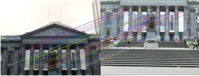
Fig. 5: Feature Matching after applying RANSAC
