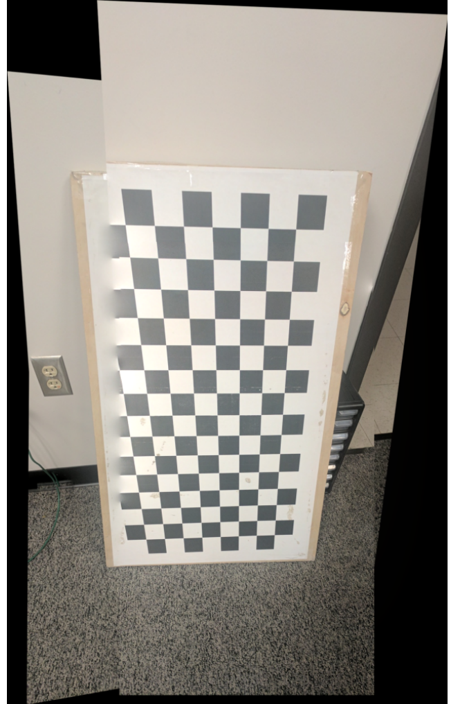
Fig. 21: Final Pano for Test Set 1. Note that the checkerboard pattern makes it incredibly difficult for the technique to find correct homographies, as features are not unique, so the result is not perfect. Despite this, the left and right halves stitched incredibly accurately.
