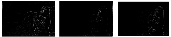
Fig. 31: Canny, Sobel, and Pb lite outputs for Image 5
