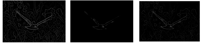
Fig. 32: Canny, Sobel, and Pb lite outputs for Image 6
