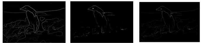
Fig. 33: Canny, Sobel, and Pb lite outputs for Image 7
