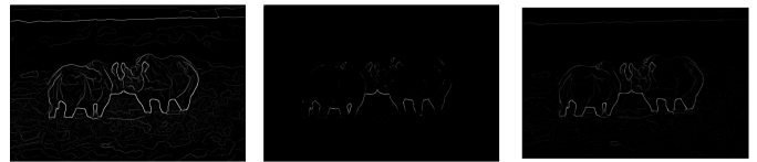
Fig. 34: Canny, Sobel, and Pb lite outputs for Image 8
