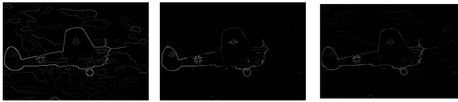
Fig. 27: Canny, Sobel and Pb lite outputs for Image 1
