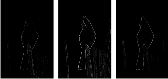
Fig. 34. Sobel, canny, PbLite outputs for image10.jpg
