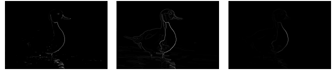
Fig. 28. Sobel, canny, PbLite outputs for image4.jpg
