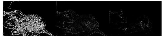
Fig. 33. Pb-Lite output, Canny output, and Sobel output for Image 9
