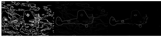
Fig. 25. Pb-Lite output, Canny output, and Sobel output for Image 1
