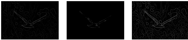
Fig. 32. Comparison of Pblite (1) with Sobel(2) and Canny(3) for Image 6
