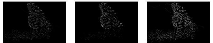
Fig. 29. Comparison of Pblite (1) with Sobel(2) and Canny(3) for Image 3
