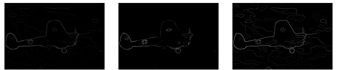
Fig. 27. Comparison of Pblite (1) with Sobel(2) and Canny(3) for Image 1
