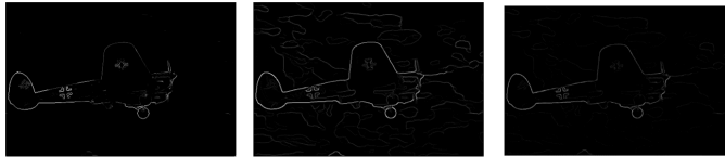
Fig. 17. Sobel, Canny, and Pb-lite output of Image 1
