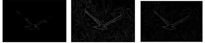
Fig. 22. Sobel, Canny, and Pb-lite output of Image 6
