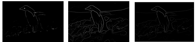
Fig. 23. Sobel, Canny, and Pb-lite output of Image 7
