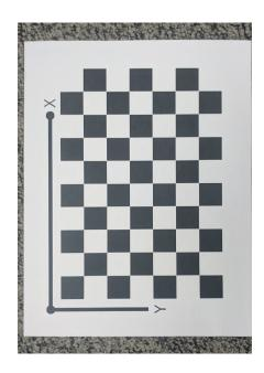
The first step is to find the pixel coordinates of the chessboard corners in each image. Points are found using the *cv2.findChessboardCorners* function. The patternsize parameter is (9,6) which is the number of inner corners that are to be detected. A total of 54 corner points are found for each image.
