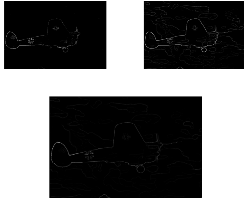
Fig. 16. Canny(top-right), Sobel(top-left) and PBLite(bottom) Outputs of Image1
