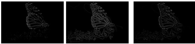
Fig. 28: Sobel, Canny, and pb-lite output of image 3.
