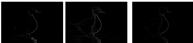
Fig. 29: Sobel, Canny, and pb-lite output of image 4.
