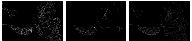
Fig. 27. Canny, Sobel and pb-lite output for Image 2
