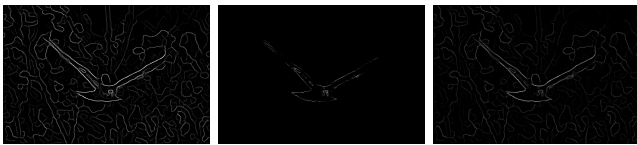
Fig. 31. Canny, Sobel and pb-lite output for Image 6
