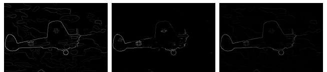
Fig. 26. Canny, Sobel and pb-lite output for Image 1
