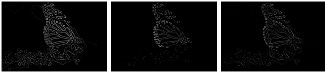
Fig. 28. Canny, Sobel and pb-lite output for Image 3
