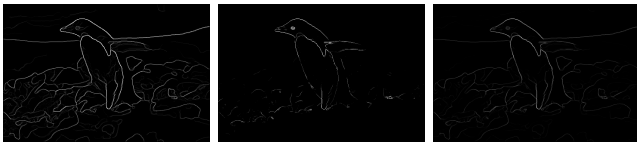
Fig. 32. Canny, Sobel and pb-lite output for Image 7
