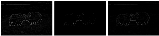
Fig. 33. Canny, Sobel and pb-lite output for Image 8
