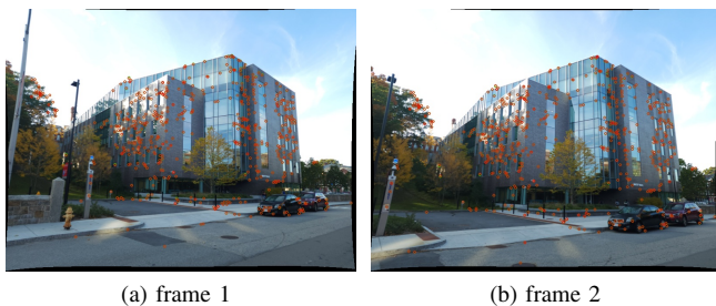
Fig. 9: Projections after BA. The first column corresponds to the first frame and the second column corresponds to the second frame. Green dots show the feature detections and red dots show reprojections.
