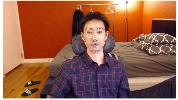
Fig. 14: Face landmark detected by deep learning method
