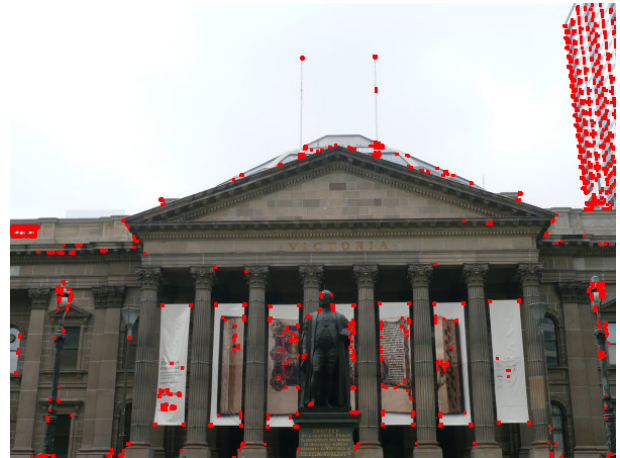
Fig. 3. Detected corners using Harris Corners method for input 1
