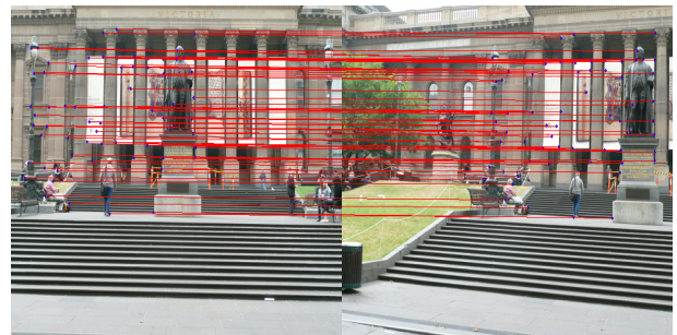
Fig. 14. Feature matches after outliers have been removed using RANSAC for input 2 and 3
