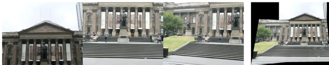
Fig. 2. First three images: Input to the panorama stitching algorithm, last image: output of the panorama stitching algorithm
