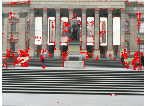
Fig. 4. Detected corners using Harris Corners method for input 2
