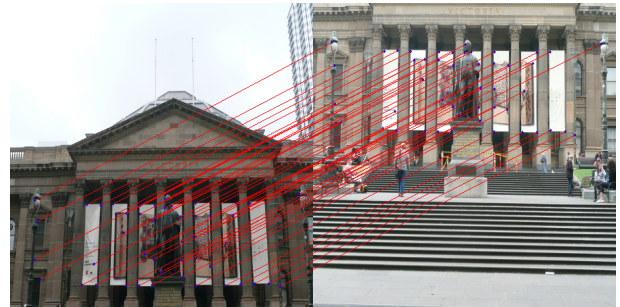
Fig. 13. Feature matches after outliers have been removed using RANSAC for input 1 and 2
