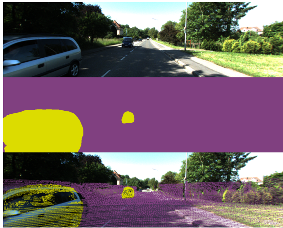
Fig. 9. Original Image, Segmented Image and the point cloud fused
