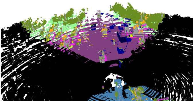
Fig. 9: Semantic Segmented Point Cloud
