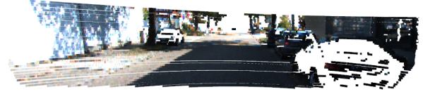
Fig. 5. Point cloud data painted using the source camera RGB images (In camera perspective).
