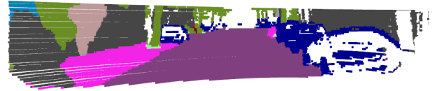
Fig. 7. Point cloud data painted using the source segmented images (In camera perspective).
