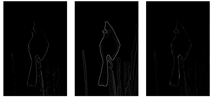
Fig. 38. Image 10 Sobel Baseline, Canny Baseline, (Ours) Pb-Lite Output
