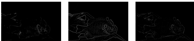
Fig. 37. Image 9 Sobel Baseline, Canny Baseline, (Ours) Pb-Lite Output
