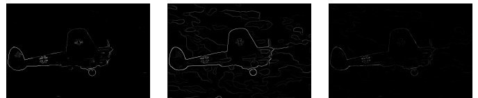
Fig. 29. Image 1 Sobel Baseline, Canny Baseline, (Ours) Pb-Lite Output
