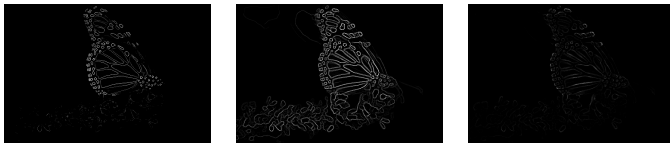
Fig. 31. Image 3 Sobel Baseline, Canny Baseline, (Ours) Pb-Lite Output
