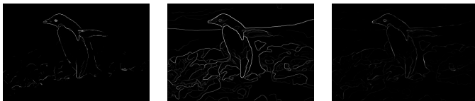
Fig. 35. Image 7 Sobel Baseline, Canny Baseline, (Ours) Pb-Lite Output
