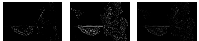
Fig. 30. Image 2 Sobel Baseline, Canny Baseline, (Ours) Pb-Lite Output
