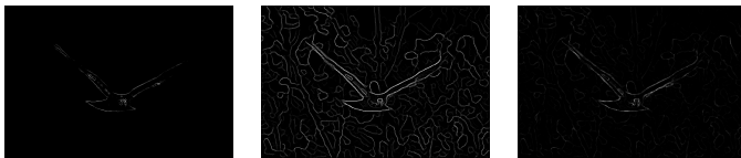
Fig. 34. Image 6 Sobel Baseline, Canny Baseline, (Ours) Pb-Lite Output
