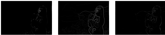
Fig. 33. Image 5 Sobel Baseline, Canny Baseline, (Ours) Pb-Lite Output
