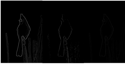
Fig. 35: Sobel, Canny, and pb-lite result of image 10
