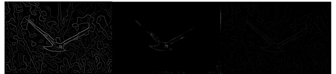
Fig. 31: Sobel, Canny, and pb-lite result of image 6
